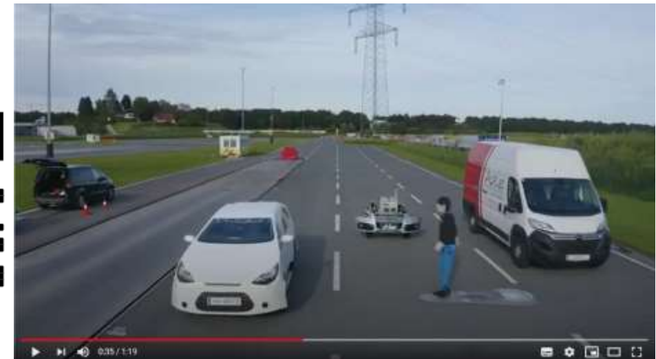
Traffic scenario testing with SPIDER and robot platforms
